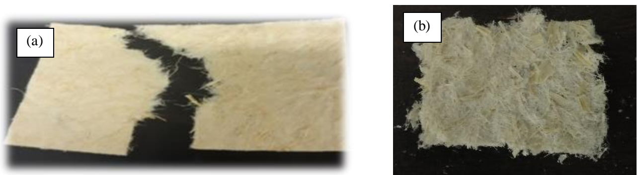
Figure 6 : Physical appearance of oil palm leaf paper processed using starch (a) and without starch (b)
